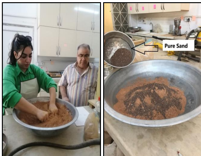
Fig 5: Preparing raw materials for brick making in the laboratory by changing the proportion of sand.
