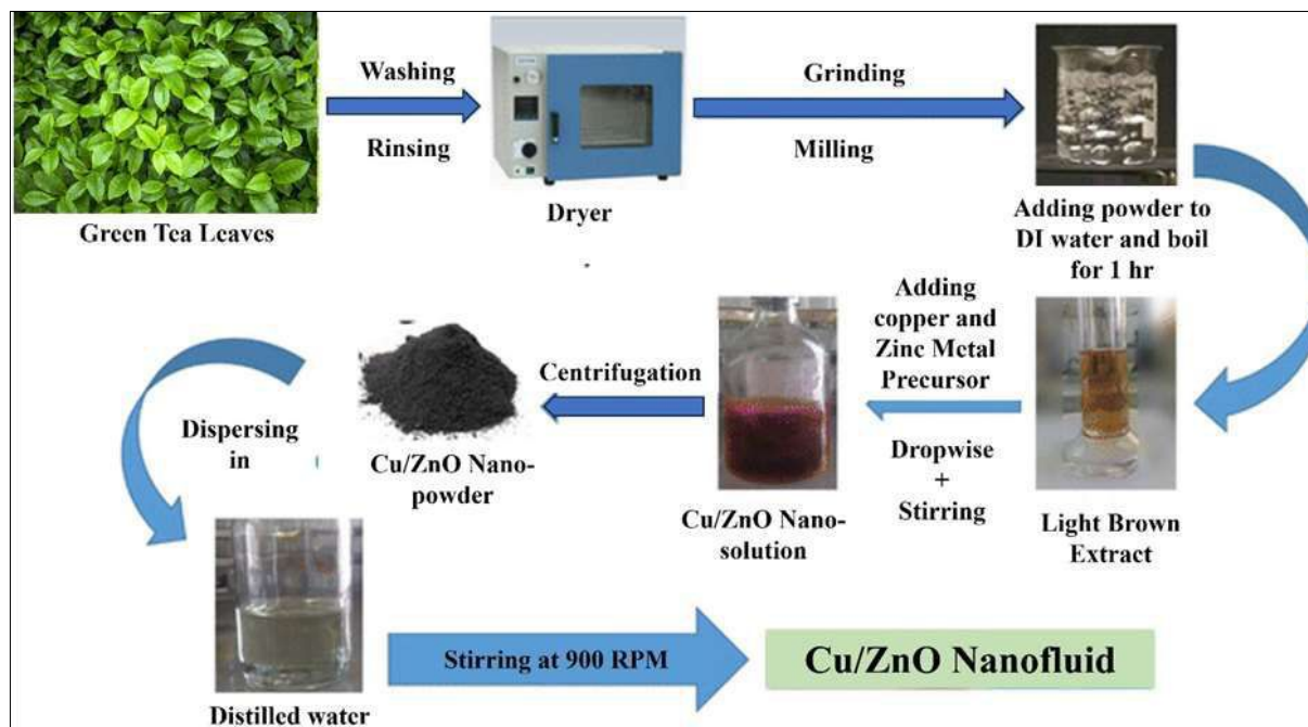
Fig 3: Preparation method of bimetallic nanoparticles
