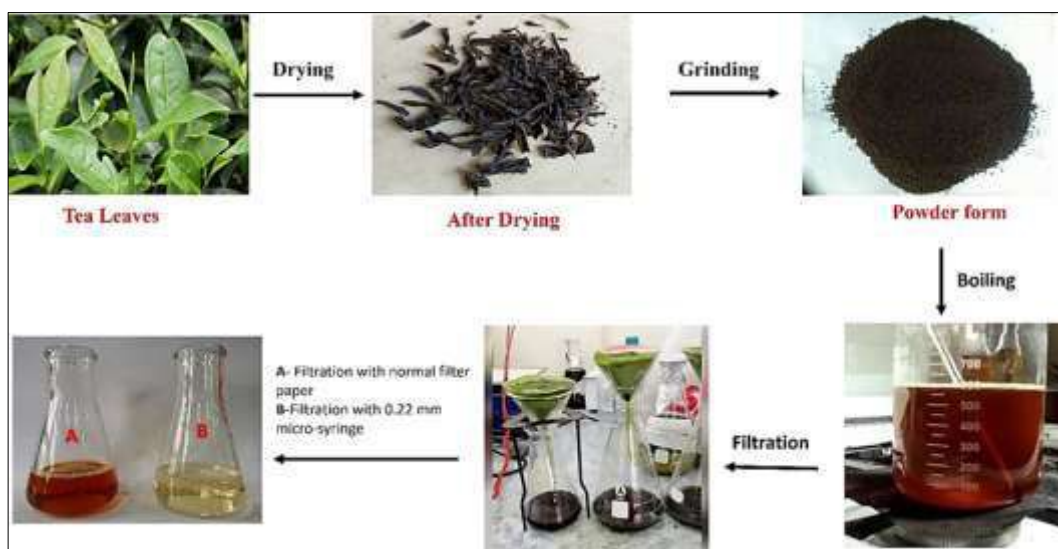
Fig 2: Plant extract preparation method
