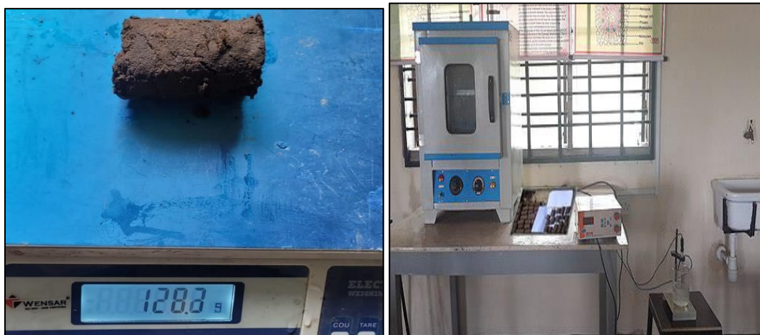
Fig 6: Measuring moisture content and weight of briquette
